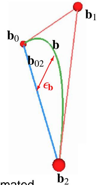
**Lemma:** Minimal distance between arcs **a** and **b** can be approximated by minimal distance between straight base line segments **a<sub>02</sub>** and **b<sub>02</sub>**:
